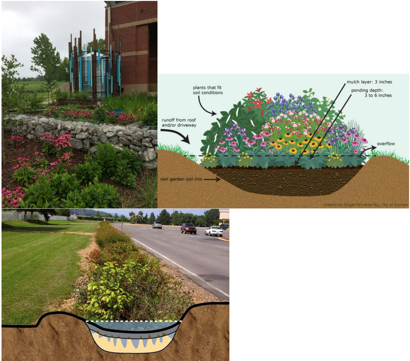
Image: Rain gardens, such as the one at the Mississippi State University Landscape Architecture Facility (left), are designed to channel and filter excess rainwater. Diagram on the right is from City of Durham, NC. Bottom shows rain garden picture overlaid with diagram of water flow, from Alabama Cooperative Extension System.
