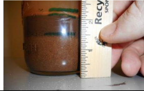
Using a ruler, measure and record the height of each layer, and the total height of all three layers. Andrew "Drew" Jeffers, ©2018, Clemson Extension
