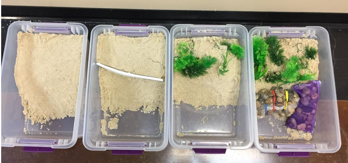
Image: From left to right, sand only, bulkhead, living shoreline with plants, living shoreline with plants and oyster reef. Image showing the complete shoreline setups.
