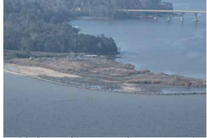
Left. A “before” picture of the northern tip of Mon Luis Island; right, an “after” picture of the same area after restoration. Sandy material was used to backfill the breakwater and planting of marsh vegetation will occur in 2017.
