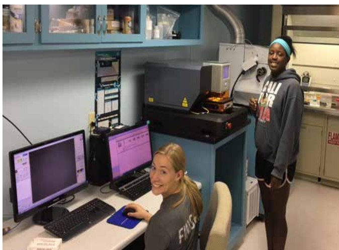
Graduate students Kayla DaCosta and Anika Knight processing samples with the laser ablation platform and inductively coupled plasma mass spectrometer.
